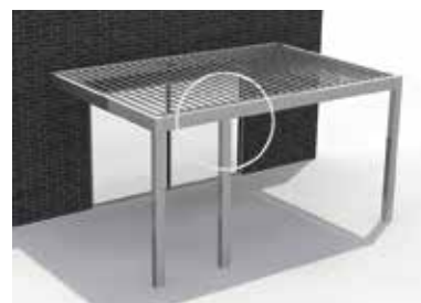
Door post under the frame
